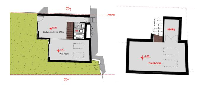
8.3 Ancillary outbuildings often benefit from permitted development rights however in this case it should be noted that the outbuilding does not conform to permitted development as the height is more than 2.5 metres within 2 metres of the boundary and has a basement and therefore planning permission is required.
